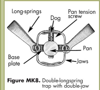
**Figure MK8.** Double-longspring trap with double-jaw
