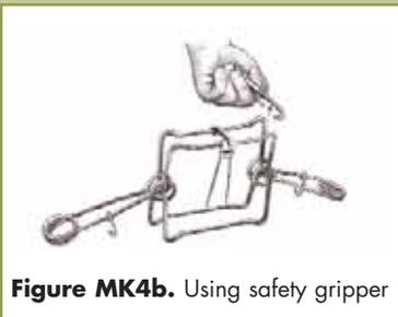
**Figure MK4b.** Using safety gripper
