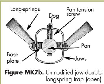
**Figure MK7b.** Unmodified jaw double-longspring trap (open)
