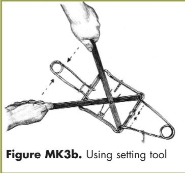
**Figure MK3b.** Using setting tool
