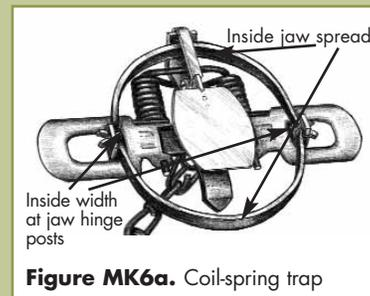
**Figure MK6a.** Coil-spring trap
