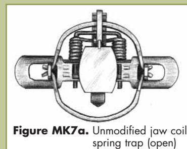
**Figure MK7a.** Unmodified jaw coil-spring trap (open)
