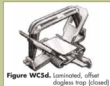
**Figure WC5d.** Laminated, offset dogless trap (closed)
